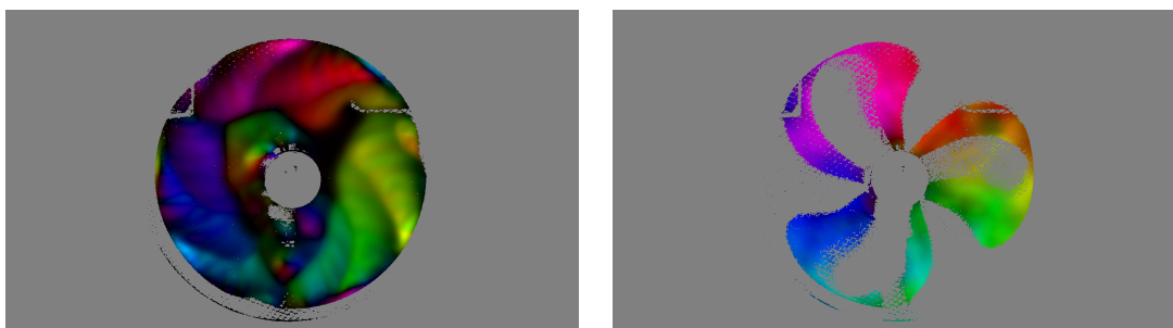
Figure 3.9 – Sample EBOF results for the Fan sequence of our high-speed dataset, with \Delta t = 15\text{ms} (left) and \Delta t = 5\text{ms} (right). Notice how the blades of the fan are merged together in the first case, while they appear clearly in the second one, leading to improved optical flow results.
